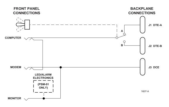
Figure 2-1. PatchSwitch with In-Line Access (PSM-01, PSM-02)
